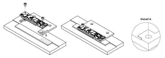
Recommended use of M2 fasteners with washers. For more information see <u>Table of recommended fastener tightening</u> torques at RLS Media center.
